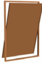
Figure 4-42 A pivoted window rotated around the vertical axis
